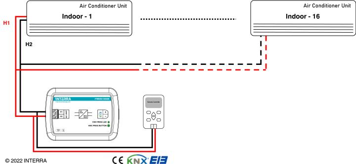
The figure on the left shows the connection diagram between the Viessman AC-KNX Gateway, air conditioner remote controller and multiple air conditioner indoor units. If more than 2 indoor units are to be connected to an air conditioner remote controller, care must be taken to ensure that the connection is as shown in the adjacent figure. Some Indoor unit models do not support multi indoor unit control.
