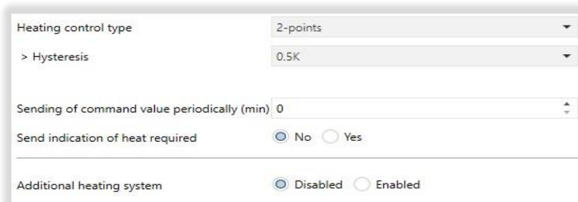
Fig. 24 : Heating 2-Points Control Configuration
